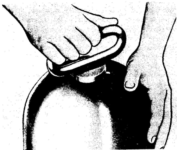
Figure 106—Installing Dome Lifting Handle
